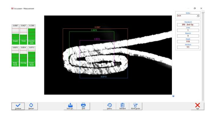
Images of the can seam can be saved for later review, and all dimensions are saved to the database for organization into reports.
