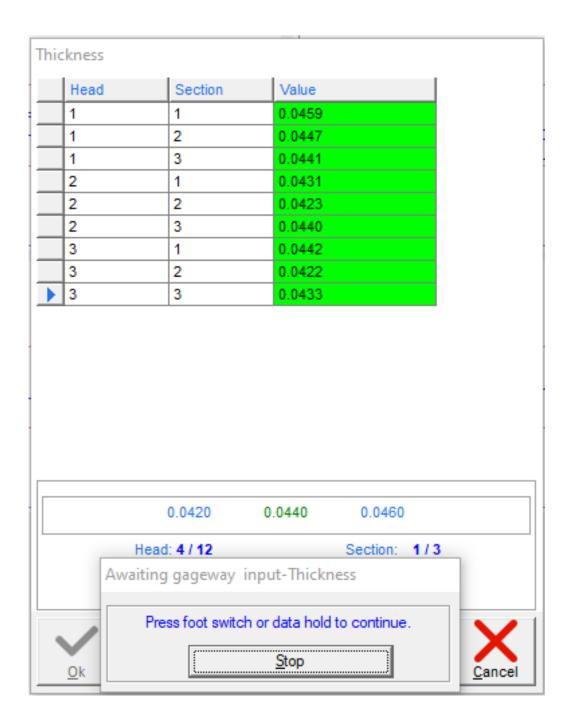
After seam thickness and countersink measurements are taken, the cans are opened, drained, rinsed, and cross sectioned with the seam saw. The HD optical unit is then used to automatically measure Seam Height, Overlap, Cover Hook, and Body Hook.
