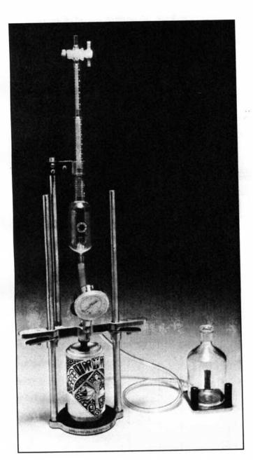
This instrument is recommended for testing air content where greater speed and accuracy is required. It is automatically adjustable to various size bottles and cans and is available in one and two litre sizes. The parts list and line drawing on page 16 of this manual should be used for assembly and as a reference when ordering replacement parts.
